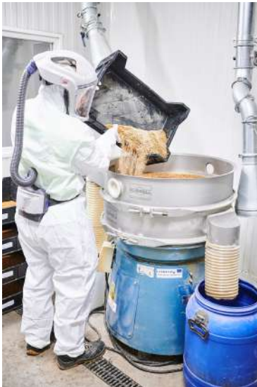
Figure 7: Full face mask and suit as protection during sieving at harvest to protect against dust and allergens.
